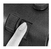
5. As the tape plays, read the script and press the slide-forward button (FORWARD) for about 1/2 second at the points indicated in the script. The tray will advance one slide as each signal is recorded. Reassuring "beeps" will be made audible when recording slide-advance pulses if the volume control is raised slightly during recording. (You won't hear the "beeps" during tape playback.)
